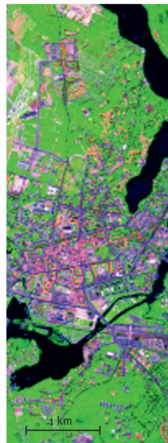
Fig. 6: Simulated EnMAP image (color composite) of the city and surroundings of Potsdam, Germany, showing various urban, agricultural, managed forest and aquatic ecosystems. The simulation is based on airborne hyperspectral image data (HyMap). EnMAP will allow a more frequent coverage of larger areas than feasible in airborne campaigns.
