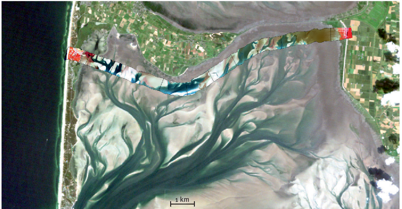
Fig. 24: Satellite image of the Wadden Sea with low spectral resolution (Landsat) in the background and a strip of high-spectral resolution airborne scanner data (AISA). This figure exemplifies the different spatial coverage of extensive landscapes like the Wadden Sea achievable with locally collected airborne data compared with region-wide satellite data.
