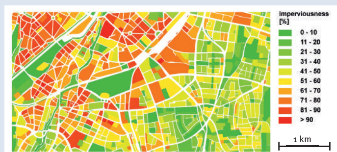
Fig. 30: Extent of ground sealing per block of buildings for the eastern part of Munich, derived from hyperspectral data.
