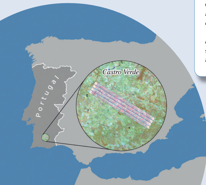
Fig. 17: Simulated EnMAP data for the Castro Verde region, Portugal. False-color representation superimposed on a Landsat-5 TM satellite image.
