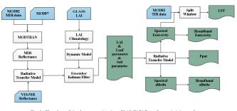
Fig. 1. Flowchart of simultaneous estimation of LAI, FAPAR, surface emissivity, surface albedo and LST by integration of optical to TIR remote sensing.
