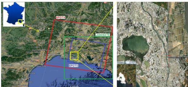
Figure 1. Location of the study area with the footprints of the remote sensing images used (SPOT4 in red, LC8 in green and SPOT 5 blue) and the vector layer of the plot boundaries.
