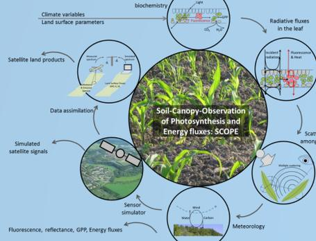
SCOPE is a vertical (1-D) integrated radiative transfer and energy balance SVAT model, with, amongst others, sun-induced chlorophyll fluorescence (SIF) and net photosynthesis of the canopy (NPC) as outputs.
