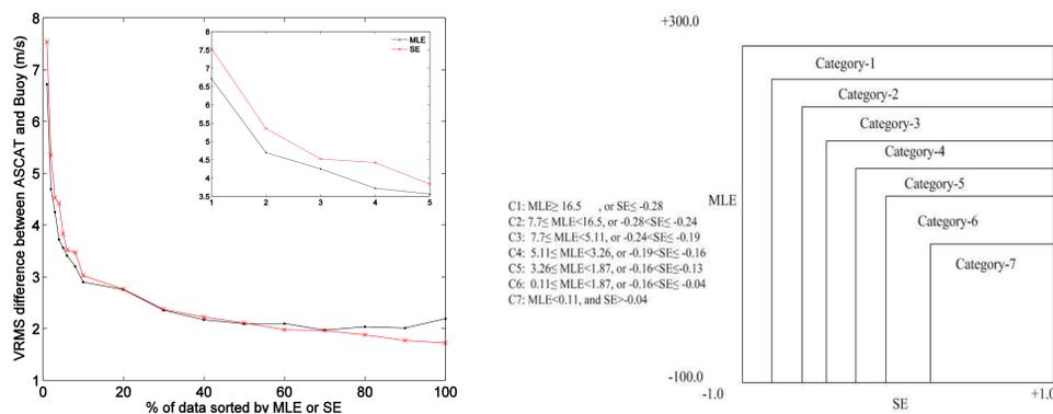
Fig. 1 The Vector Root-Mean-Square (VRMS) difference between ASCAT (25-km product) and buoy winds as a function of the percent of data sorted by MLE (in descending order) and SE (in ascending order). A zoom of the first 5% of data is shown on the right-upper corner.
