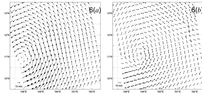
Fig. 6 (a) ECMWF forecast surface winds collocated with the ASCAT observation on July 3<sup>rd</sup> 2015, around 11:45 UTC; (b) ASCAT-derived wind ambiguities; the lower-left reference scale indicates two opposite ambiguities with the same speed of 10 m/s.
