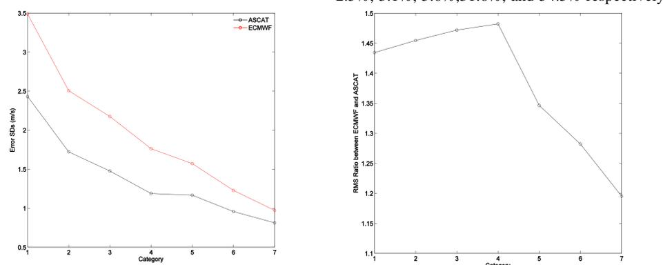
Fig. 3 Root-Mean-Square (RMS) error (the average of the random errors associated with wind  $u$  and  $v$  components, i.e.  $\sqrt{\frac{SD_u^2 + SD_v^2}{2}}$ ) on the ECMWF scale for ASCAT and ECMWF winds.
