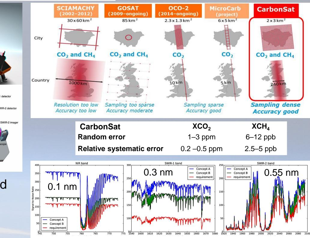
Modelled signal-to-noise spectra of the three bands and their spectral resolution
