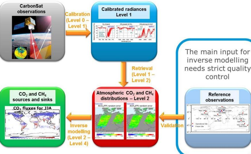
Data processing chain from CarbonSat observations to calibrated spectra, to level-2 and science products
