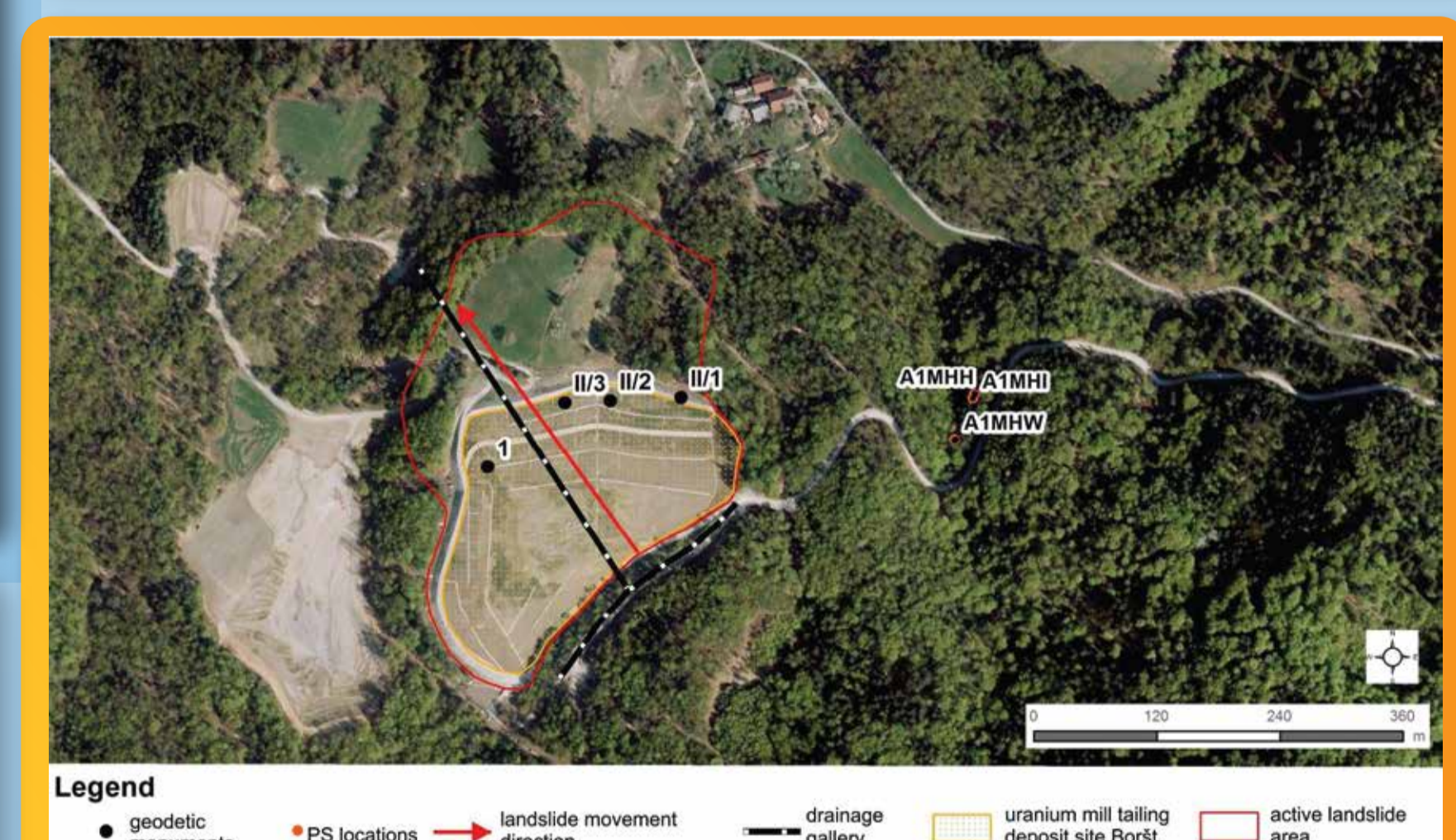
Figure 5: Landslide at uranium mill tailing deposit site Boršt
