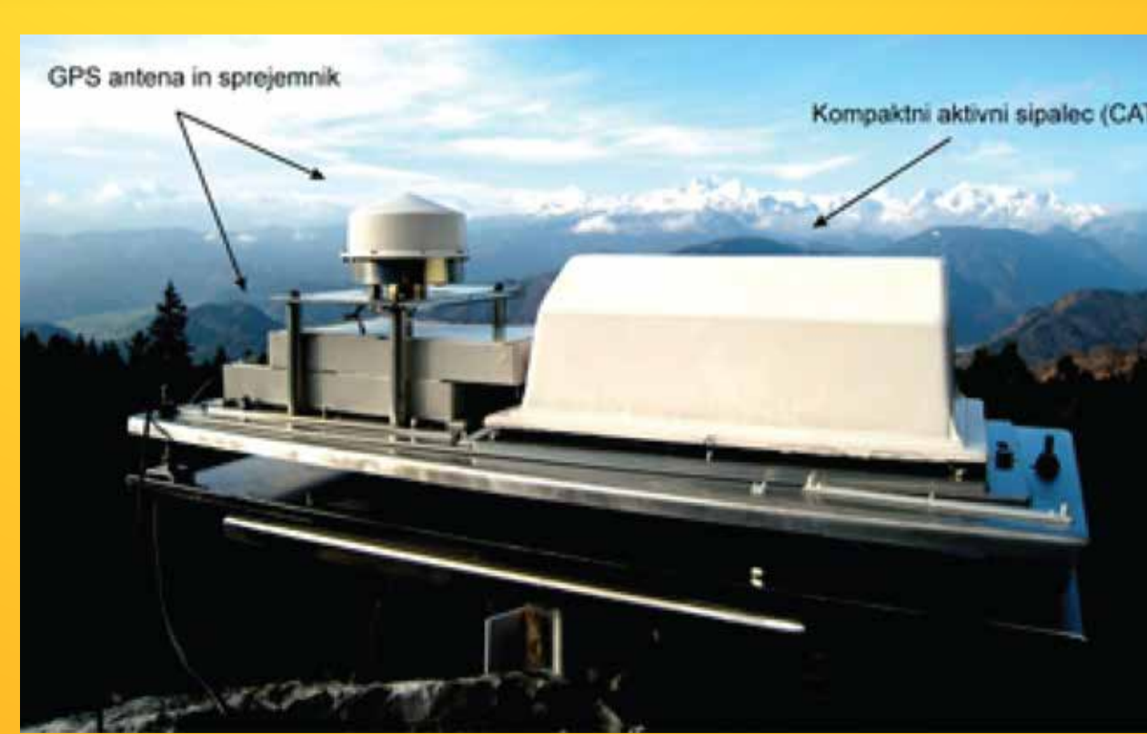
Figure 7: I2GPS instrument, a combination of GPS and CAT, installed on Potoška planina
