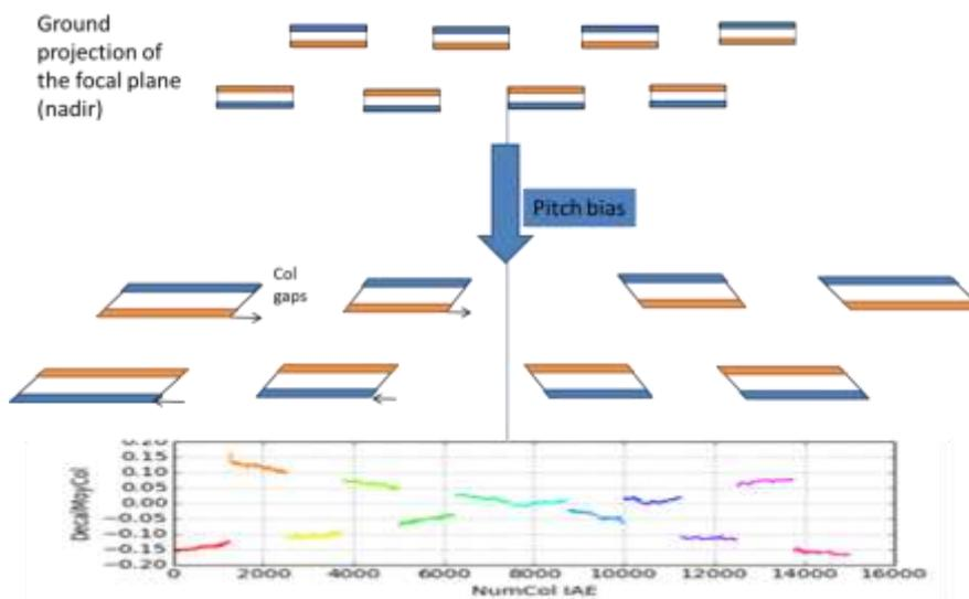
So, with a big bias update, new LOS calibration has to be done. Same kinds of effects are seen with yaw bias, or roll bias. The effect is smaller on registration when the B/H between channels is smaller. There is also an effect on absolute calibration which should be done again when a big bias is put (this should not happen again).
