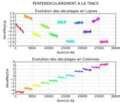
Figure 8 : first absolute focal plane cartography with geometric model defined before launch – each color is one retina
