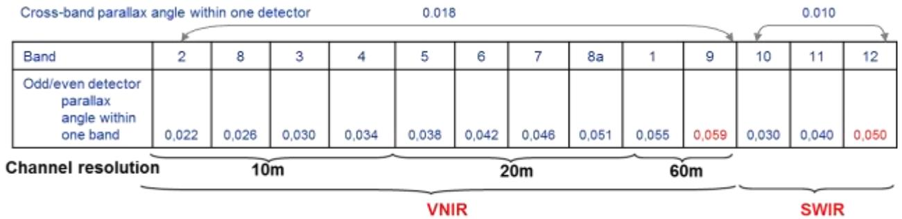
Figure 2. Parallax angles for each band, each detectors.
