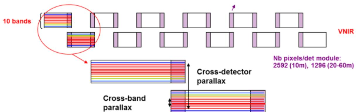
Figure 1. MSI VNIR focal plane, including 12 staggered detectors modules and ten spectral bands.
