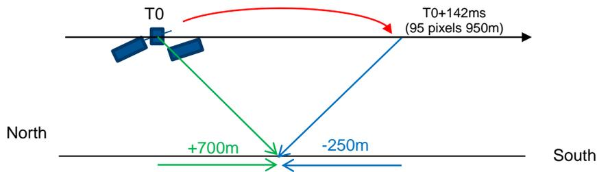
Figure 4 : biases to correct the geometric model
