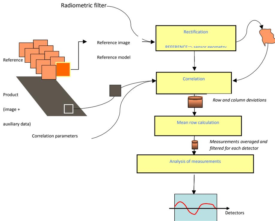
Figure 7. Detailed method for mapping the focal plane
