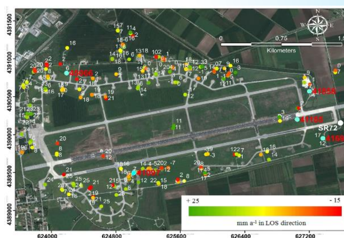
Figure 3. Average LOS velocity image along the runway and areas of Larissa National Airport for the period 1995 to 2006. The image has been saturated at ±0.1m/year-1 for visualization purposes. The numbers besides the PS candidate points indicate persistent scatterers. The borehole SR72 is shown in white and the PS candidate points used in Figure 5 are in cyan.
